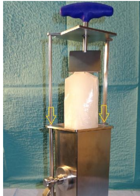
Figure 6: ice-block retainer in correct position
