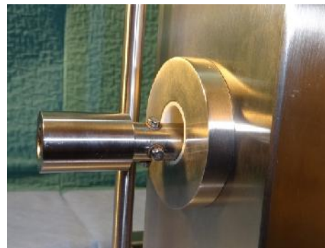
Figure 4: driveshaft in cutting-unit
