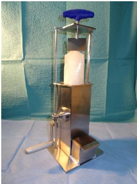
Figure 1: Atomicer with crank for manual usage
