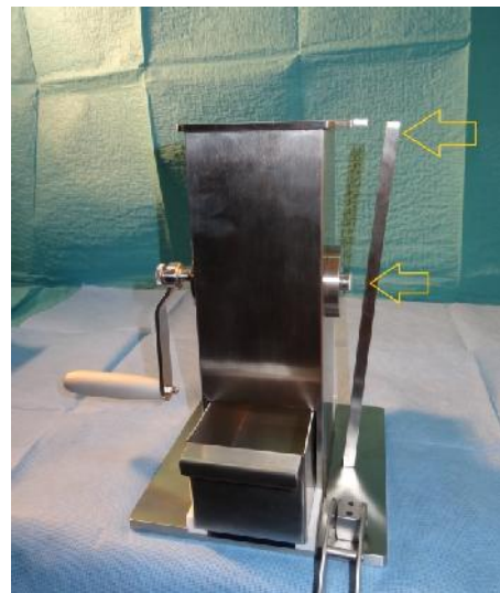
Figure 7: out swung stopper rod & driveshaft in freewheel
