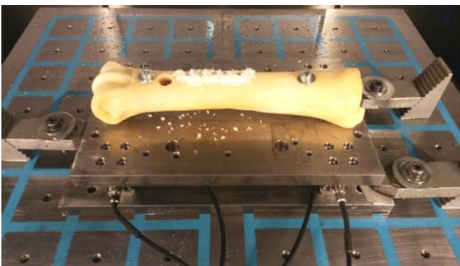
Figure 2 – Drilled bone by Hermle CNC milling machine
