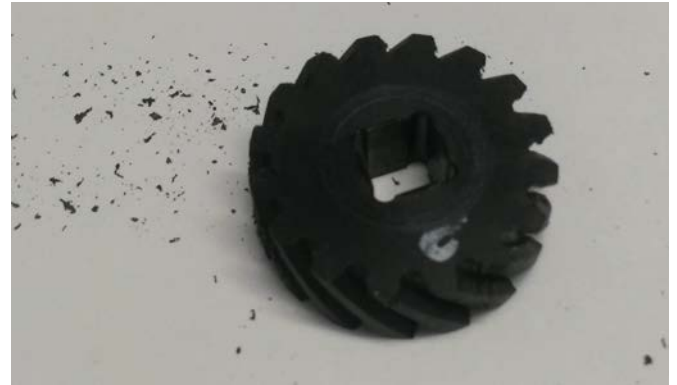
Figure 14 – Separated particles during wear experiments
